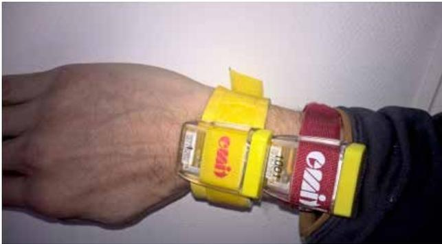
In speed the punching is performed by holding the emiTag 20-50 cm from the control for a short moment. Stretch out your hand with the emiTag toward the control and hold your hand still on top of the control unit until you have past the control.
