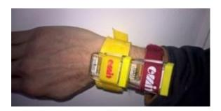
Punching is performed by holding the emiTag 0-50 cm from the punching unit at the control for a short moment. The LED light in the emiTag will start flashing and keeps flashing for 5 seconds after the punch. It is important to see this flashing, since this is the only feedback telling you that the punch is performed correctly!
